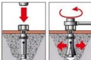
Hammer the enclosed dowels so that they are flush with the floor.
