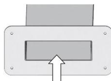
Thread the connection cables from the bottom through the column upwards through the cable opening
