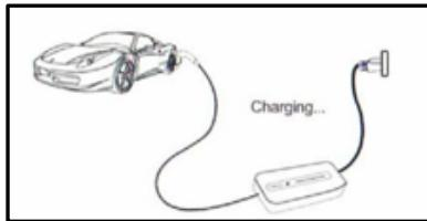
**End of Use:** Unplug the charging gun, then disconnect the power, and cover the charging gun with its cap.
